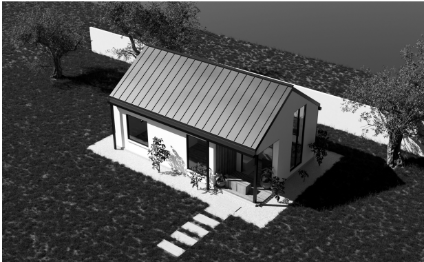
D Aerial Standing seams at 18" on center.
